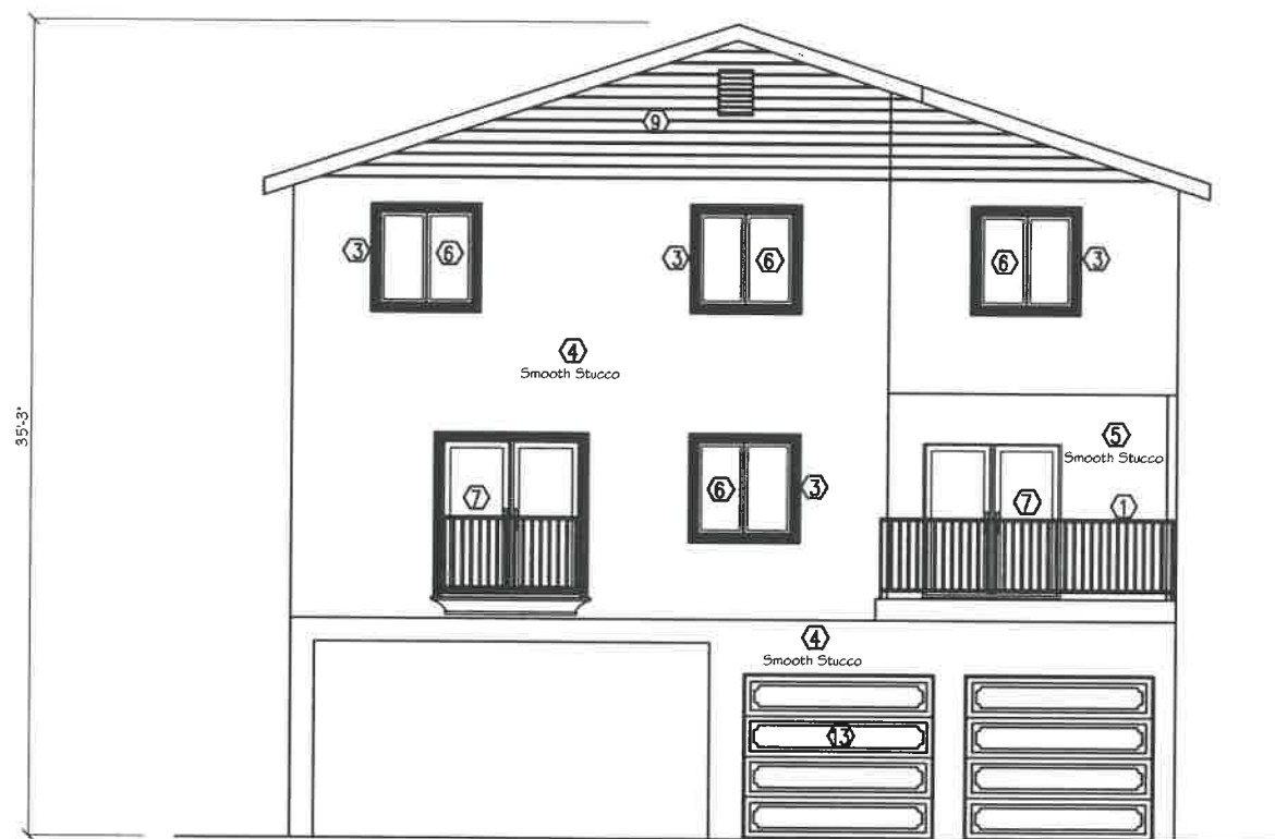
BUILDING "A" EAST ELEVATION SCALE: 1/4" = 1'-0"
