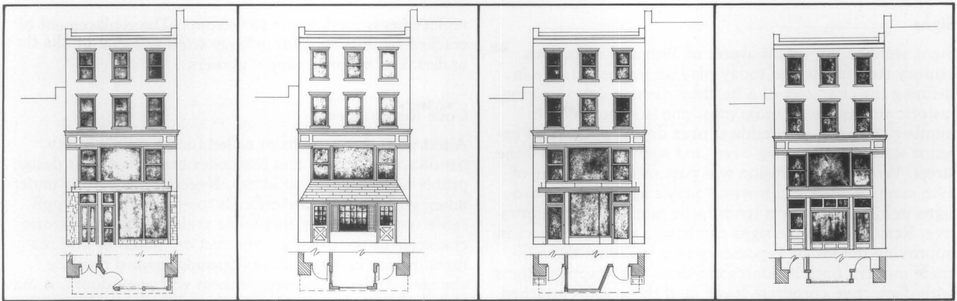
Figure 10. (A) This existing storefront, added in the 1950's to a late 19th century brick building, extends beyond the plane of the facade; faced with anodized aluminum and permastone, it does not contribute to the architectural and historic character of the building. (B) This replacement design uses "lumberyard colonial" detailing, such as barn-type doors, shutters, small paned windows, and a wood shake pent roof. The design, detailing, and choice of materials are clearly inappropriate to this commercial building. (C) This replacement design retains the 1950's projecting canopy but symmetrical placement of the doors relates well to the second floor windows above; this contemporary design is compatible with the scale and character of the building. (D) This replacement design accurately restores the original appearance of the building; based on historical research and physical evidence, it too is an acceptable preservation approach. Drawings: Sharon C. Park, AIA
