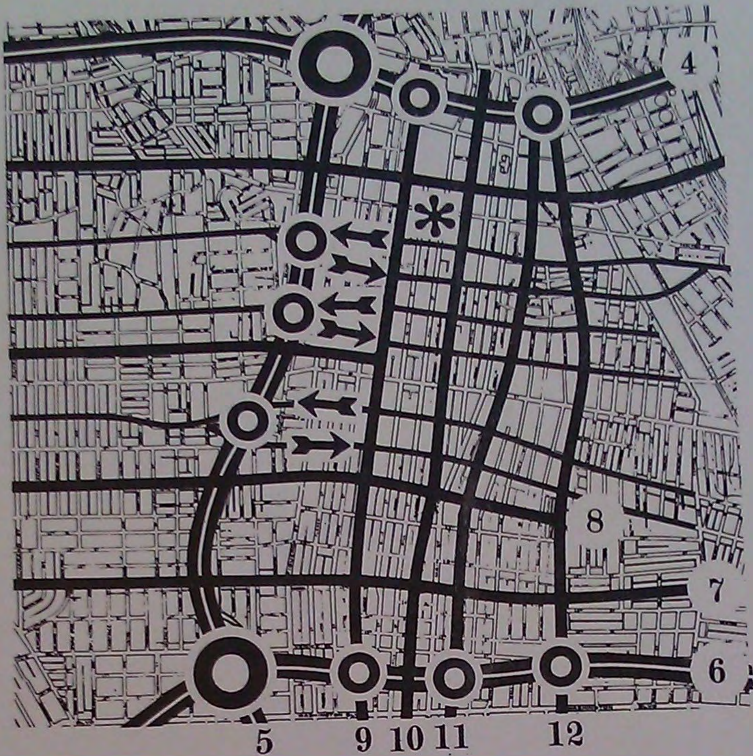
Plan of basic trafficways, free-ways and major highways in the Downtown area. Note the significance of Broadway and First Street as major traffic carriers to the four points of the compass.
