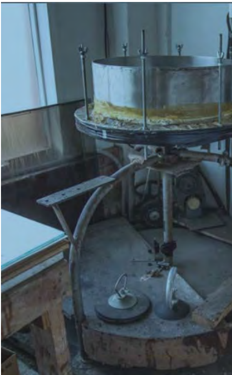
Figures 15-16 First known 20" diameter centrifugal vertical axis spin casting mold tool, built by Eversley in the studio in 1970
