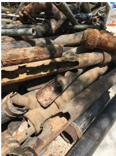
Figure 34 Old plumbing once removed from residence, showing poor condition, 2017. Photo credit: Stuart Gulland
