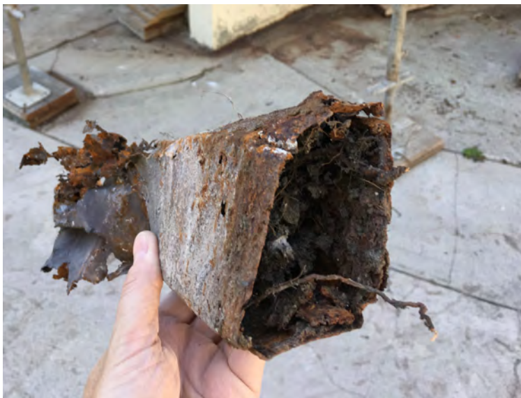
Figure 10 Portion of gutter, showing deterioration, 2017. Photo credit: Stuart Gulland
