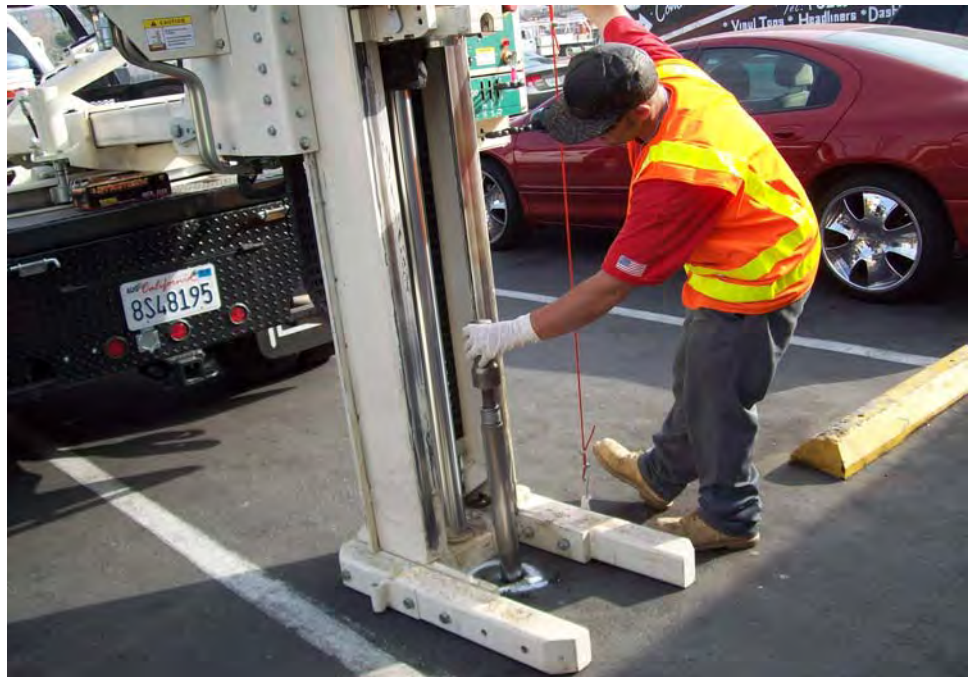
Photograph No. 3: SAE drilling soil boring B11 using a Geo Probe™ 6600
