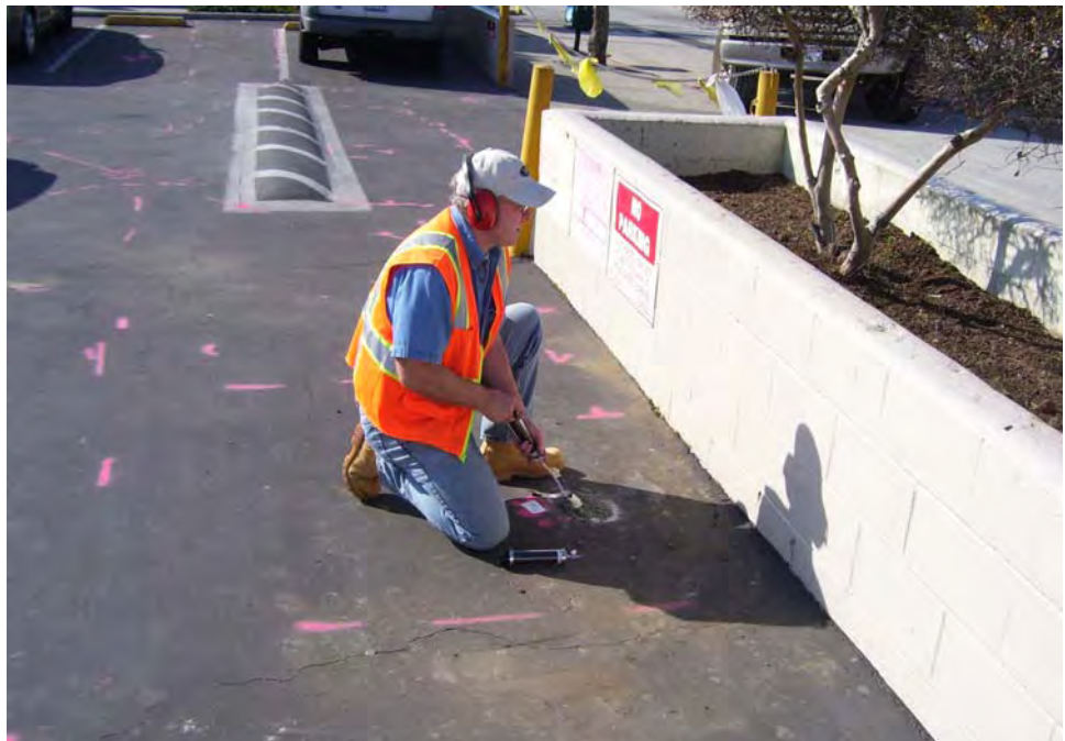
Photograph No. 6: Jones Environmental collecting Soil Vapor Sample at soil boring B1.
