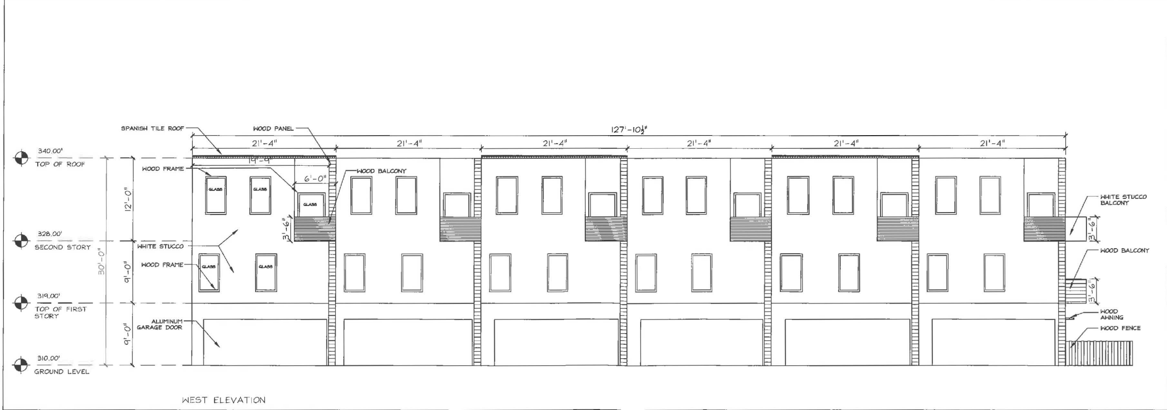
1" RECESS FOR ALL WINDOWS WEST ELEVATION SCALE: 1/8" = 1'-0"
