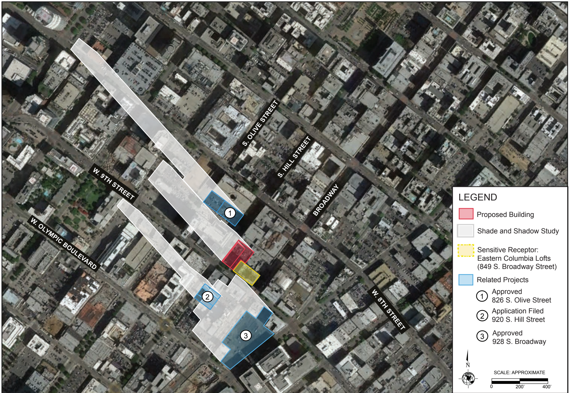
Figure III-27 Cumulative Winter Solstice Shadows 9:00 A.M.
