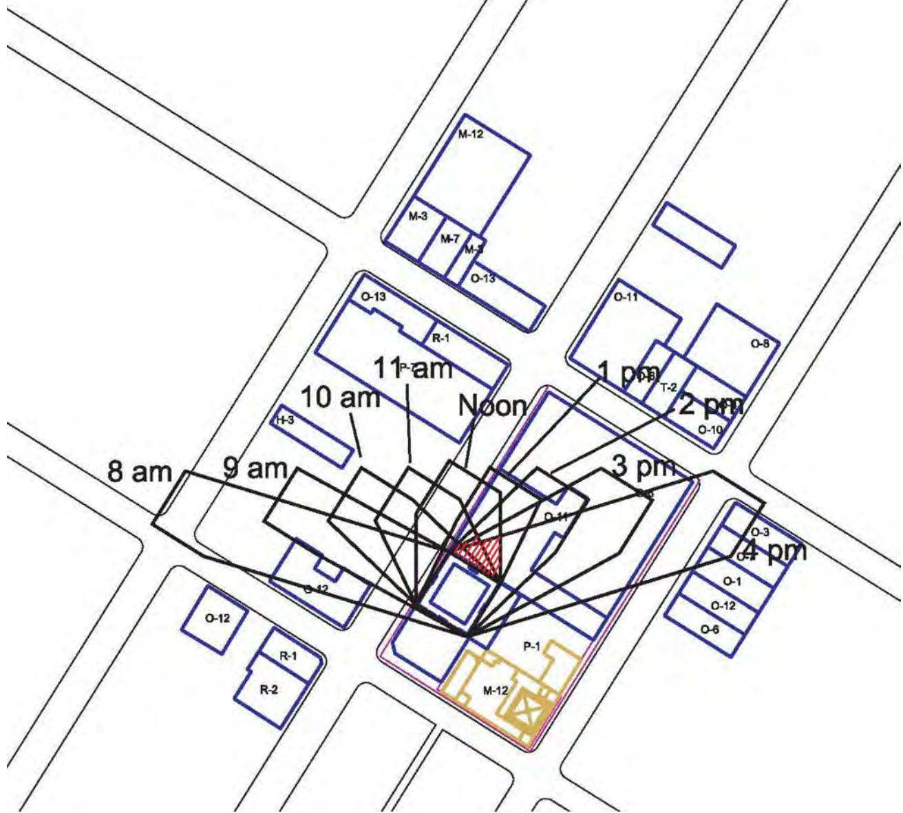
Figure III-6 Original Project - Spring - Fall Equinox Shading Diagram - Tower
