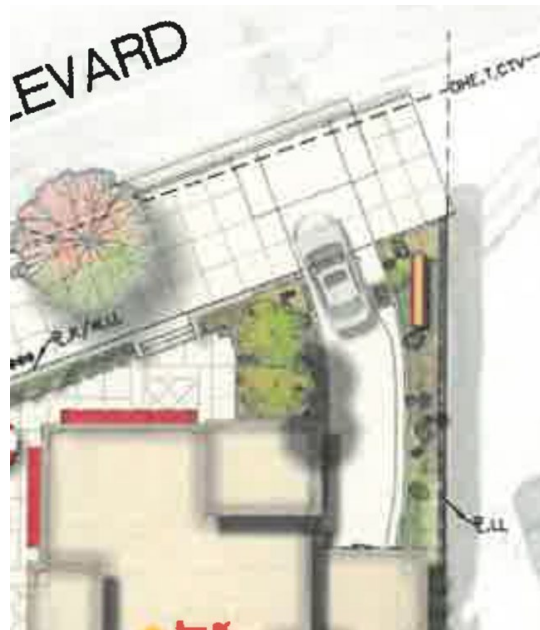
FIGURE 2 – CLOSE-UP SHOWING CAR MUST PULL ONTO SIDEWALK BEFORE DRIVER HAS LINE OF SIGHT OF POTENTIAL PEDESTRIANS ON THEIR RIGHT-HAND SIDE GIVEN LOCATION OF WALL AND SIGNAGE
