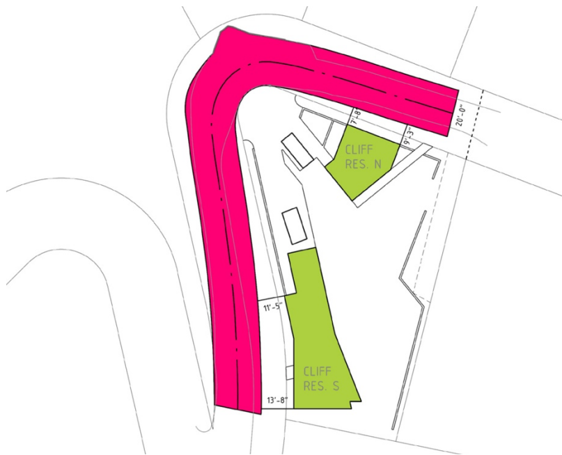
Figure 2: As dimensioned, the structures and retaining walls stand 7'-8" to 13'-8" from the edge of pavement, not at the roadway edge.
