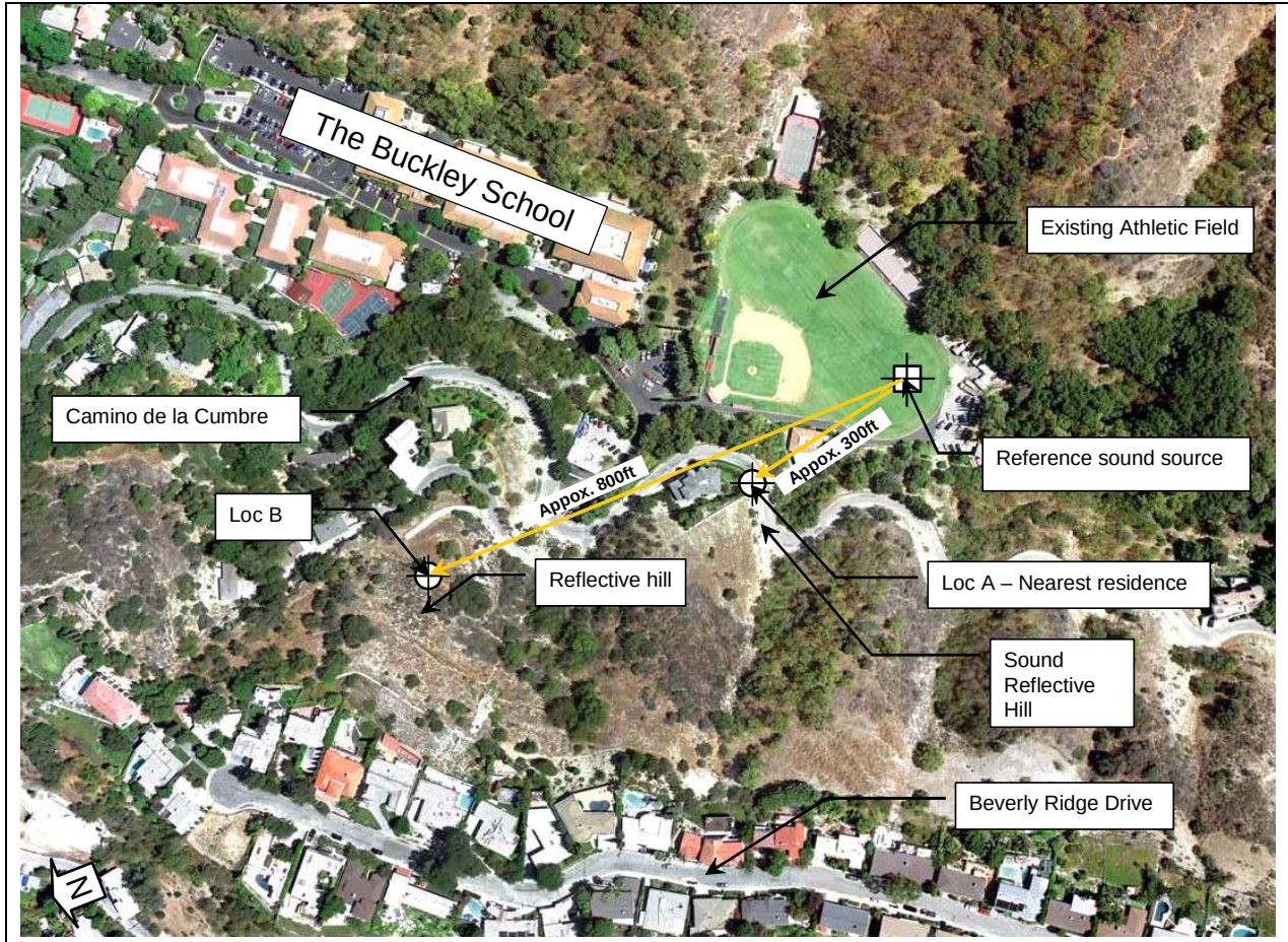
Figure 3 – Aerial Photo Showing Sound Test Configuration
