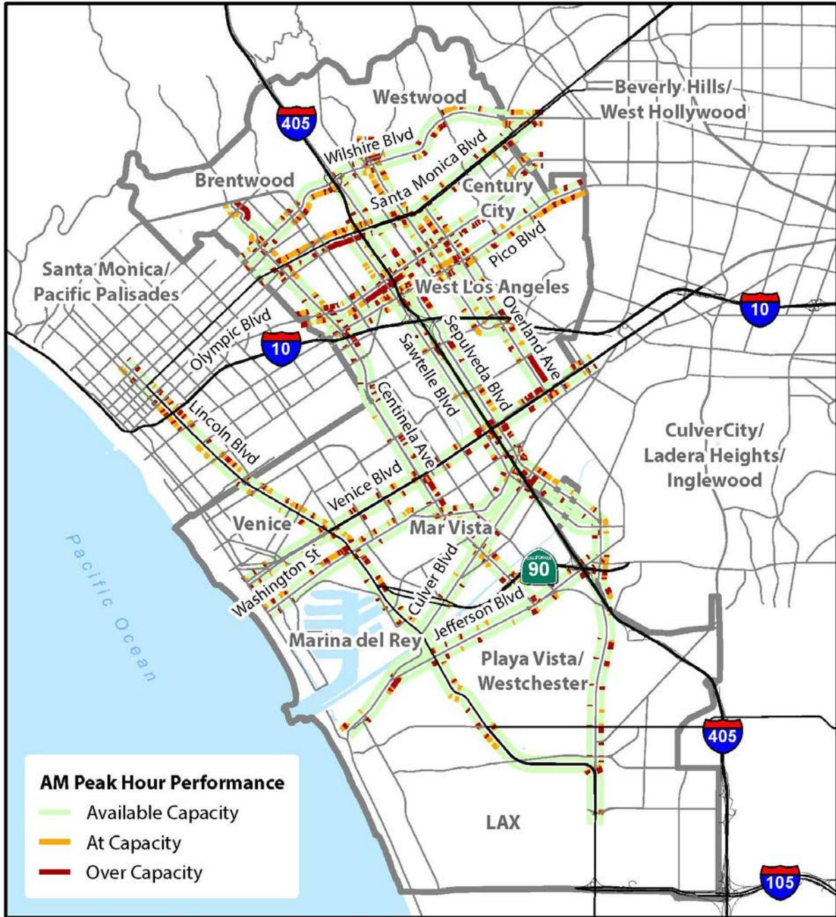
Figure 4.6-12A Corridor Operations during AM Peak Hour
