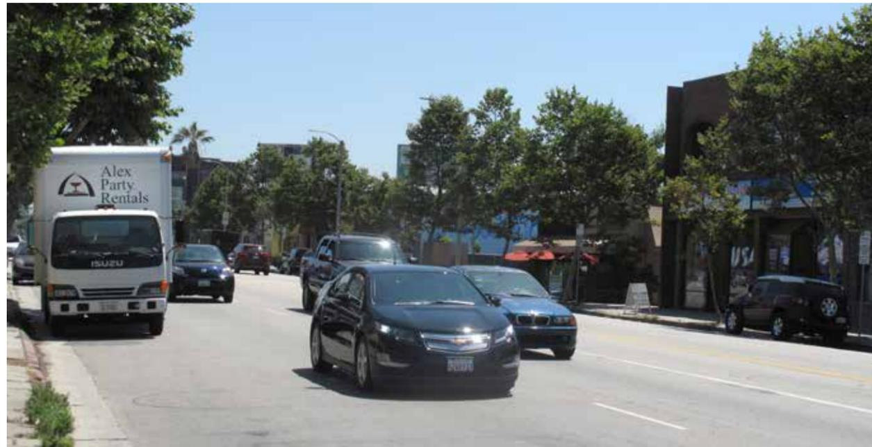
The roadway is typically 70 feet wide with two travel lanes and full-time on-street parking in each direction with a continuous center turn lane, which can accommodate medians in some midblock locations. Buildings are typically one or two story commercial storefronts with entrances along the sidewalk and limited parking behind. Some segments have more street trees than others.
