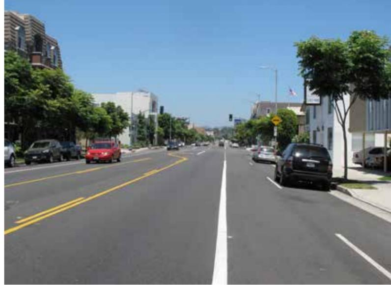
The 62-foot wide roadway accommodates one travel lane, a seven-foot wide bike lane and curbside parking in each direction with a two-way left-turn lane.
