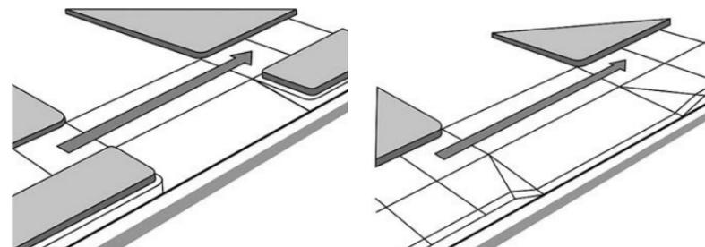
The goal of this plan is to maximize the level area of the driveway and to minimize the sloped area and align it with the parkway, unless the sidewalk is 10' wide or narrower. Image source: ITE *Designing Walkable Urban Thoroughfares: A Context Sensitive Approach* at ITE.com.
