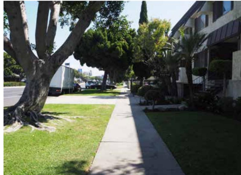
Sidewalks are 20 to 26 feet wide. Adjacent to residential uses, walkways are typically 4 feet wide and the remainder of the sidewalk is parkway.
