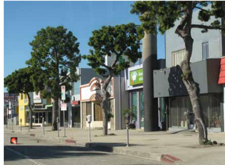
In the commercial blocks, the entire sidewalk is paved, except at small tree wells, which are setback from the curb.
