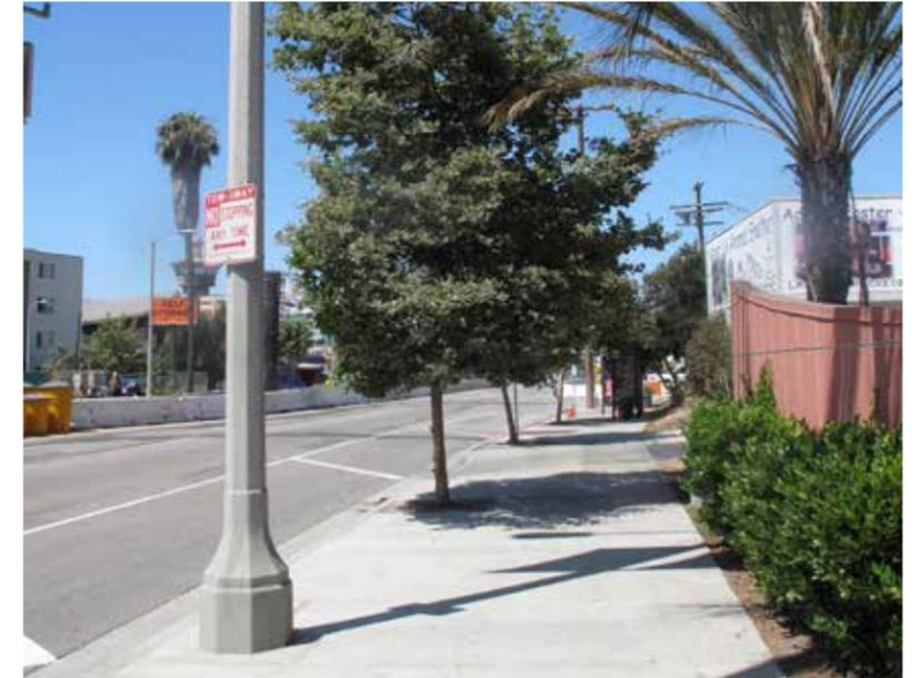
Adjacent to new commercial development, very small (4' x 4') tree wells are currently required. In both new configurations, there is little or no opportunity for infiltrating runoff from the sidewalk, so it runs off into the street.
