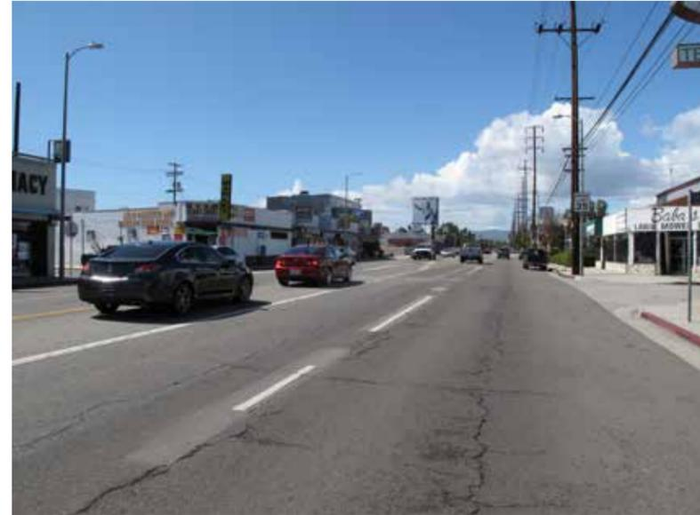
in the commercial district between Short Avenue and Culver Boulevard the roadway is 66' wide with two travel lanes and on-street parking in each direction and left-turn lanes in the center.
