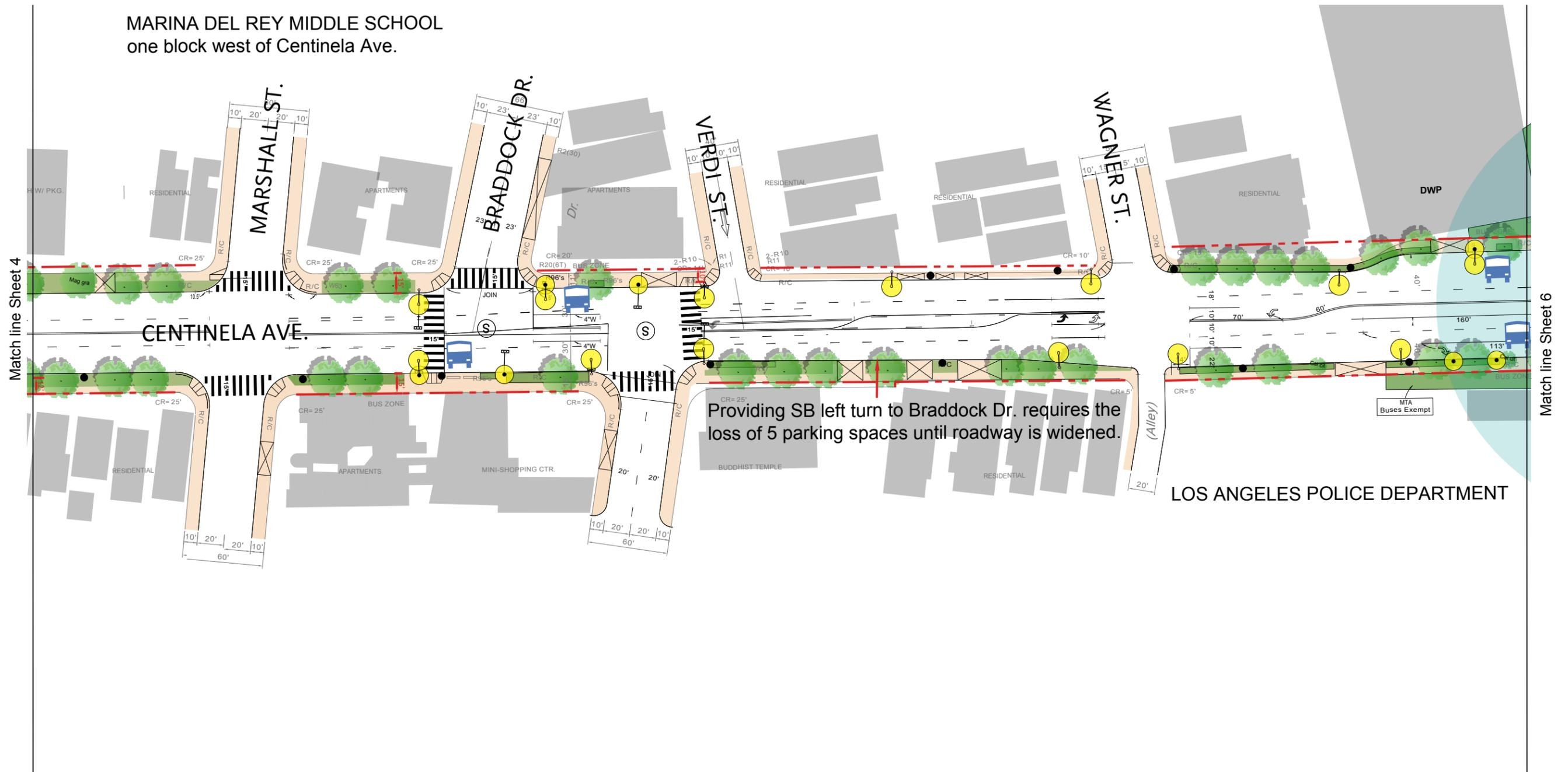
Providing SB left turn to Braddock Dr. requires the loss of 5 parking spaces until roadway is widened.
