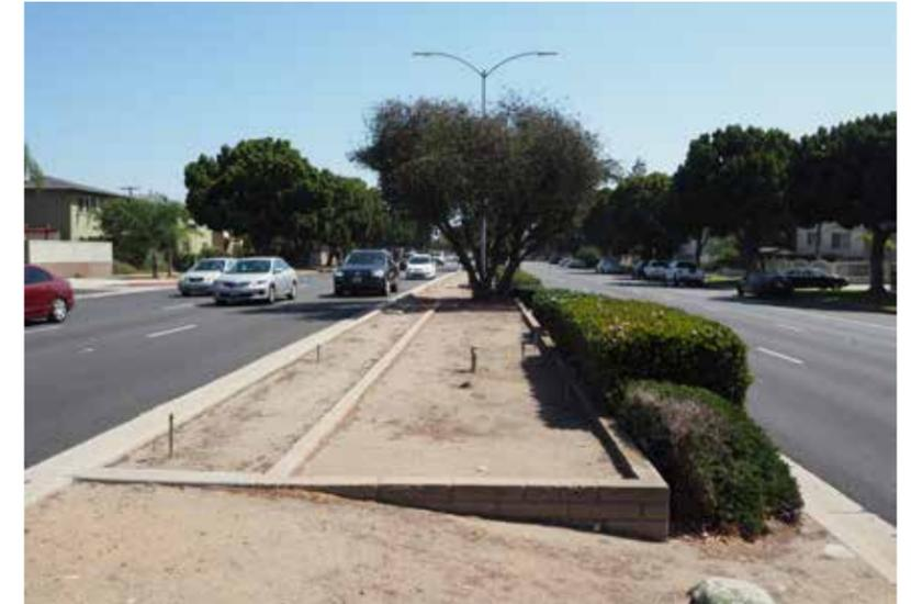
In some locations west of Centinela Avenue, there is an elevation change of 12 to 22 inches between the two sides of the median, which is accommodated by a low retaining wall..
