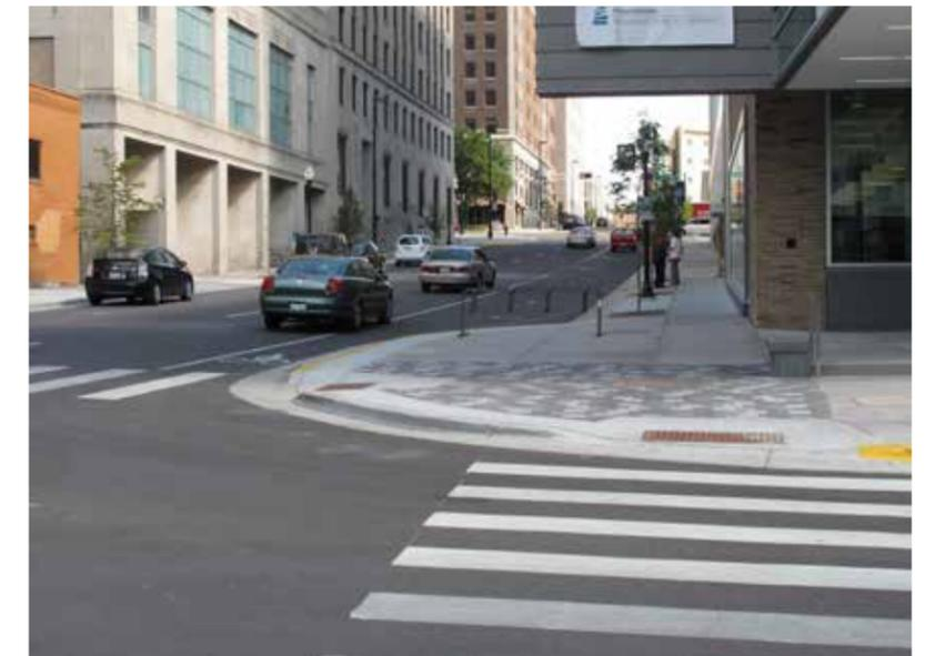
This corner has curb extensions, directional ramps and special paving for enhanced visibility and identity.
