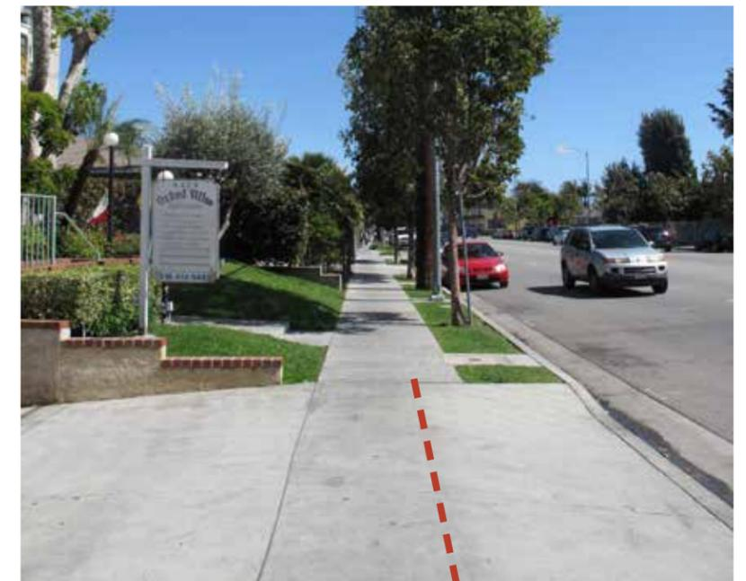
Where the sidewalk is only 10' wide, as on recently widened portions of Centinela Avenue, the maximum slope allowed by S-440 (10%), will result in the sloped portion of the driveway approach encroaching into the walkway zone.
