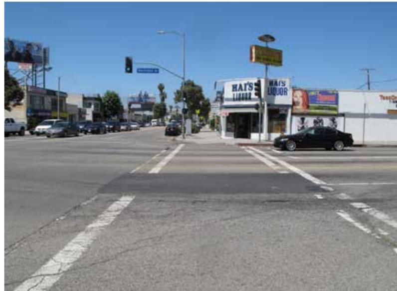
Crosswalks at signalized intersections are striped with a single white line on either side. Over time they will be converted to the City standard, Continental striping.
