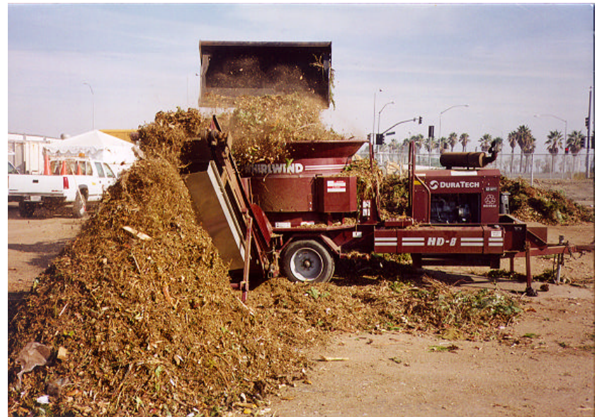
City Yard Trimmings-Grinder Operation
