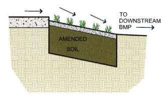
vegetation and thatch layer in the form of shallow, uniform flow. Filter strips are primarily used to pretreat runoff before it flows to an infiltration BMP or another biofiltration BMP.
