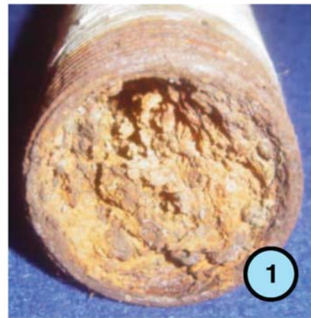
Detail of clogged and rusted pipes from the Pool Repair sketch—an example of the problem at Granada Hills
