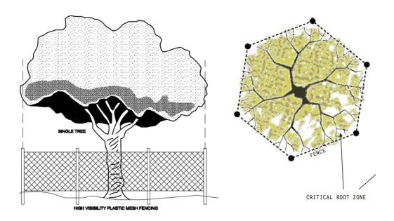
Tree protection fencing must be installed at the edge of the Tree Protection Zone (critical root zone) or beyond prior to the start of any clearing, grading or other construction activity. If space limits the fencing, place at the furthest possible distance from the trunk.
