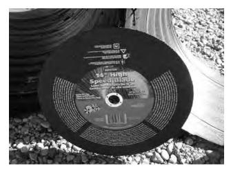
2. Blade thickness should be no less than 1/8" thick and is recommended to be made of 2-ply material that is used to cut ductile iron pipe.
