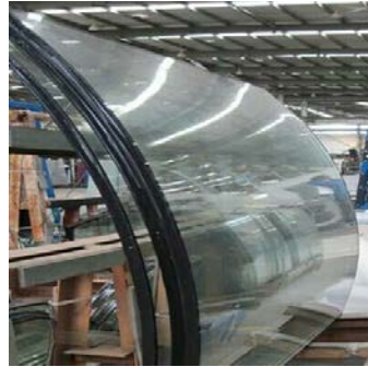
GLAZING #2: VISION GLASS, CURVED IGU, LOW REFLECTIVE
