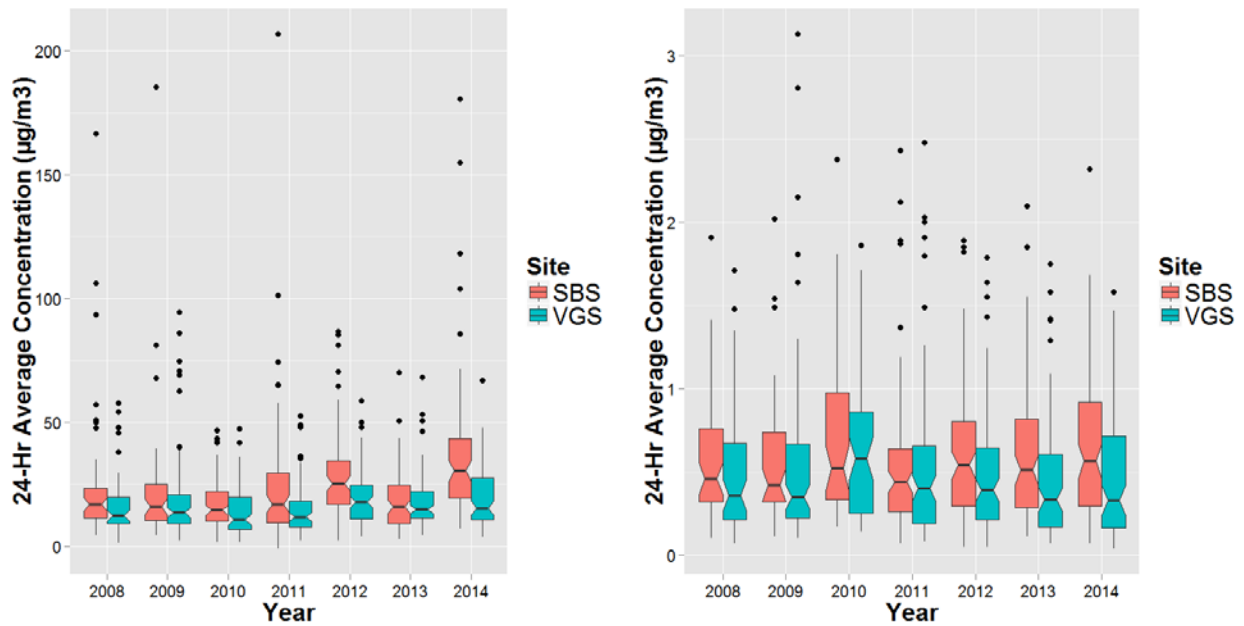
Figure 1. Notched box-whisker plot of daily 24-hr average concentrations for PM 10 (left) and BC (right) during winter season at Sunshine Canyon Landfill (SBS) and Van Gogh (VGS) in years 2008 to 2014.
