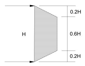
7.20.18 Where a combination of sloped embankment and shoring is utilized, the pressure will be greater and must be determined for each combination. Additional active pressure should be added for a surcharge condition due to sloping ground, vehicular traffic, or adjacent structures and must be determined for each combination.
