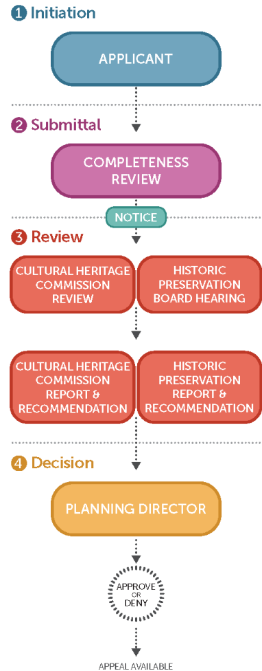
Sec. 13B.8.5. Certificate of Appropriateness (Construction)
