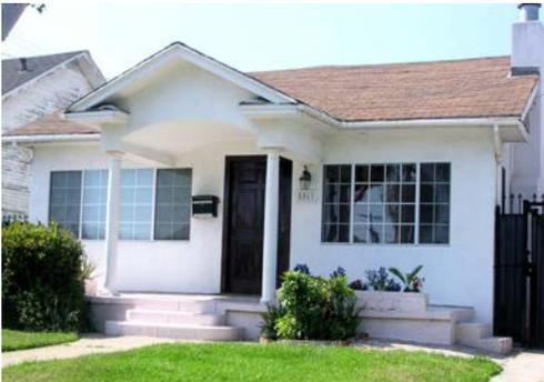
*These replacement windows are inappropriate. When putting new windows on the front facade of a home, the new windows should match the historic windows in size, shape, arrangement of panes, materials, hardware, method of construction, and profile.*
