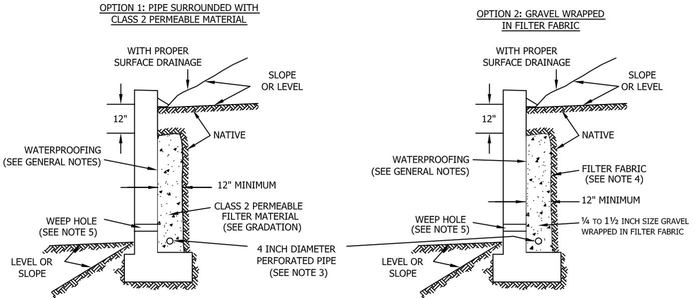
Class 2 Filter Permeable Material Gradation
