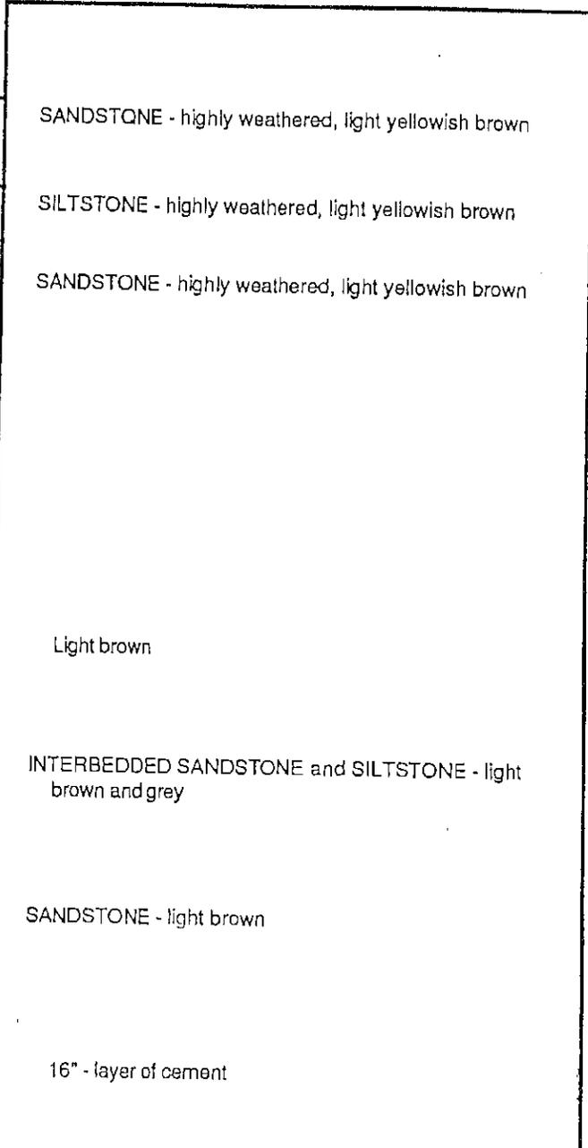
NOTE: Drilling mud used in drilling process. Mud removed after completion of drilling. Water level measured at 10' 20 minutes after completion of drilling. Boring grouted with cement.
