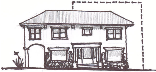
An addition in the dotted area above would be inappropriate because it would break the side facade and roof line of the house.
