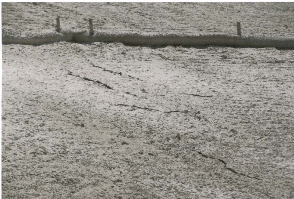
Photo 4: Cracks in Posi shell cover
