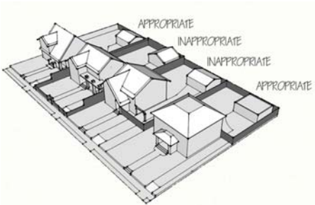
The fence arrangements in the middle two properties fortify the entire yard, obscure views of the building's features and are considered inappropriate.
