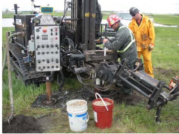
Figure 14- Waste sampling using a Sonic drilling unit
