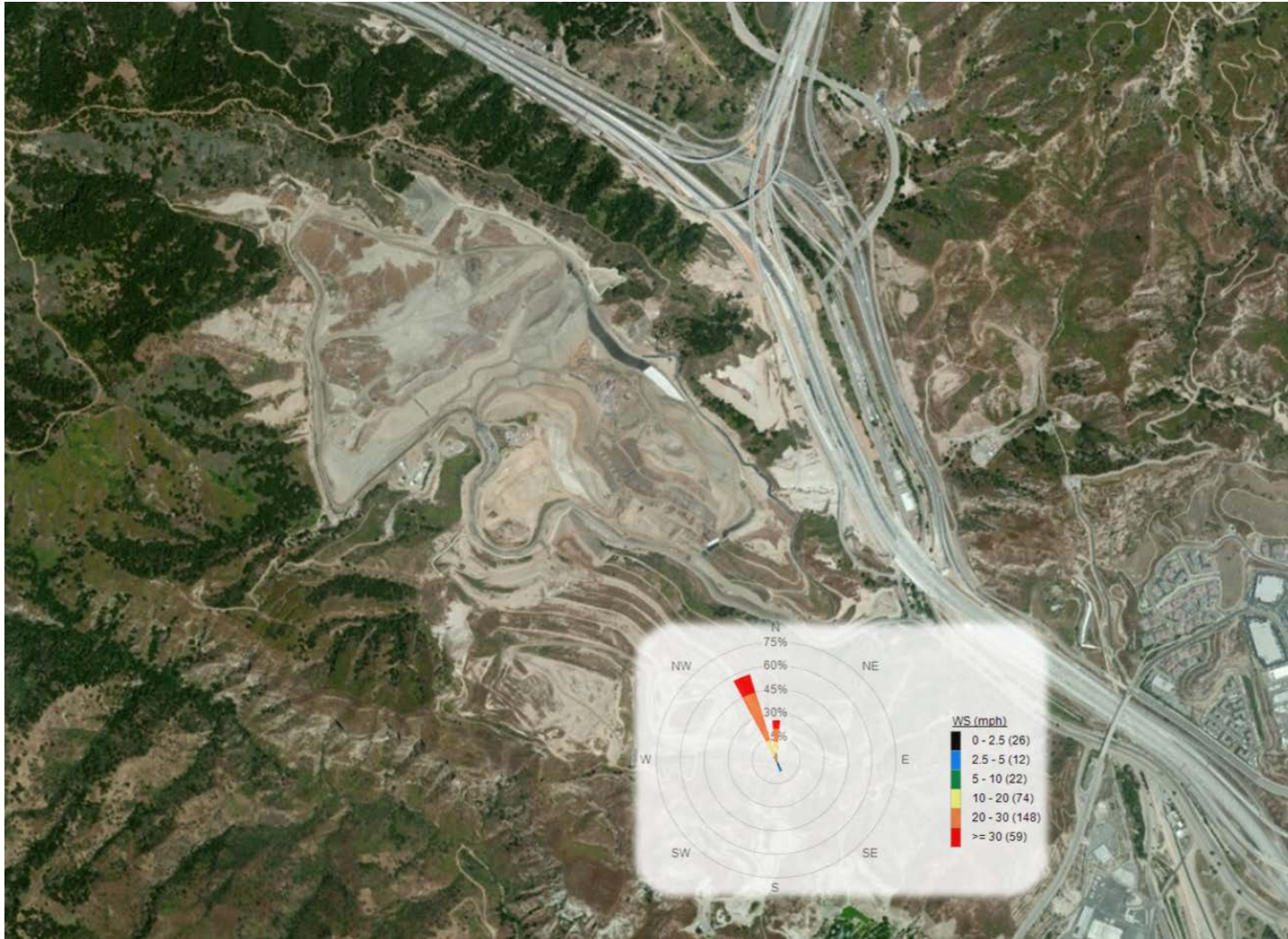
Figure 3-1. Wind rose from exceedance days during seven continuous monitoring years at the Landfill monitoring site, illustrating the fetch that encompasses working portions of the landfill. Wind speed units are mph. The wind rose center point is directly over the location of the landfill monitoring site.
