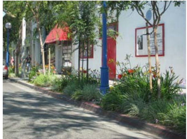
IMAGE B: Parkway can be designed to filter stormwater runoff from the street. If there is a raised curb around the parkway as in this example, the convenience strip next to the curb must be wider than 18 inches.
