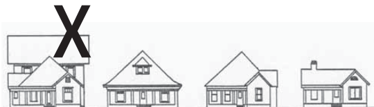
A complex roof form with many gables should not be simplified. Additions should never overpower the original structure, and should have the same roof form.
