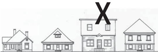
The bulk and massing of the second story, flat roof addition is out of scale with the other houses on the block.
