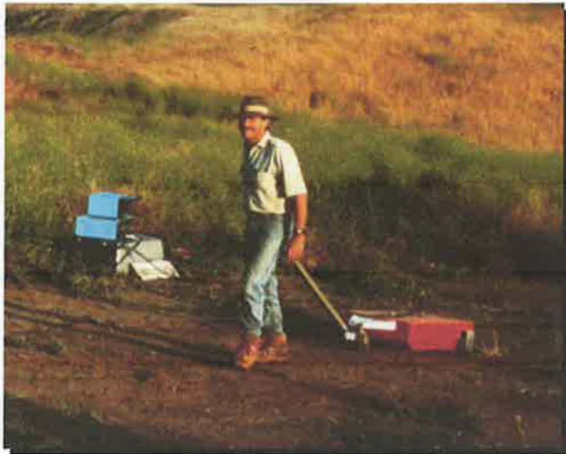
GSSI SIR-10A GPR Unit
