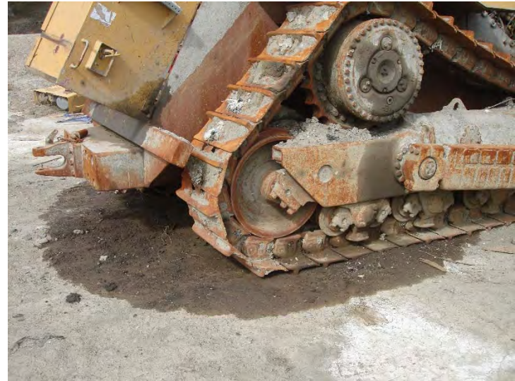
Photo 38: Equipment Leaking Oil Near Basin A: October 28, 2015
