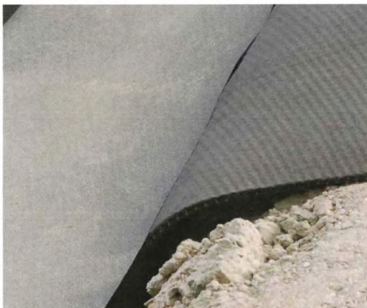
Photo 2: Geocomposite gas collection layer under liner
