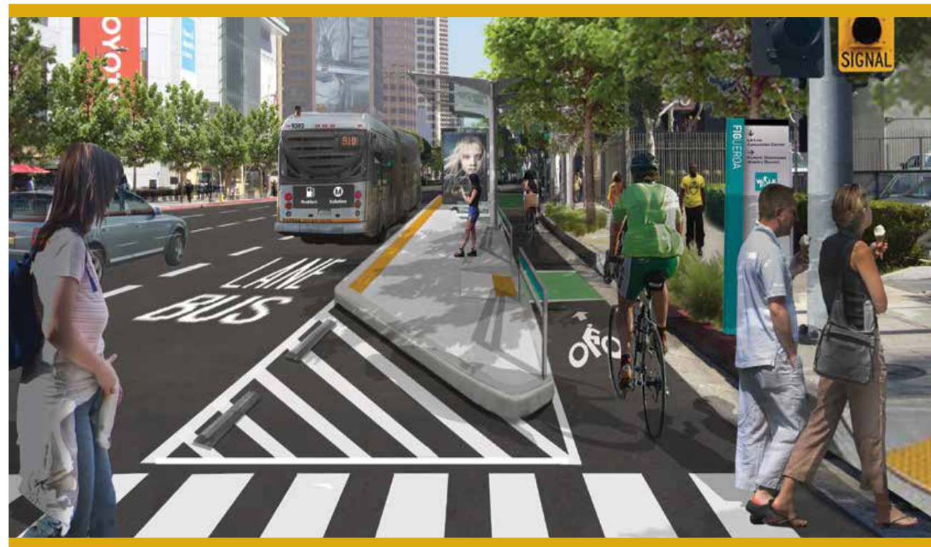
Figure D.1 above shows an example of a transit platform as illustrated in the plan for MyFigueroa. The illustrative plan to the right shows a typical protected bike lane for Crenshaw Boulevard.
