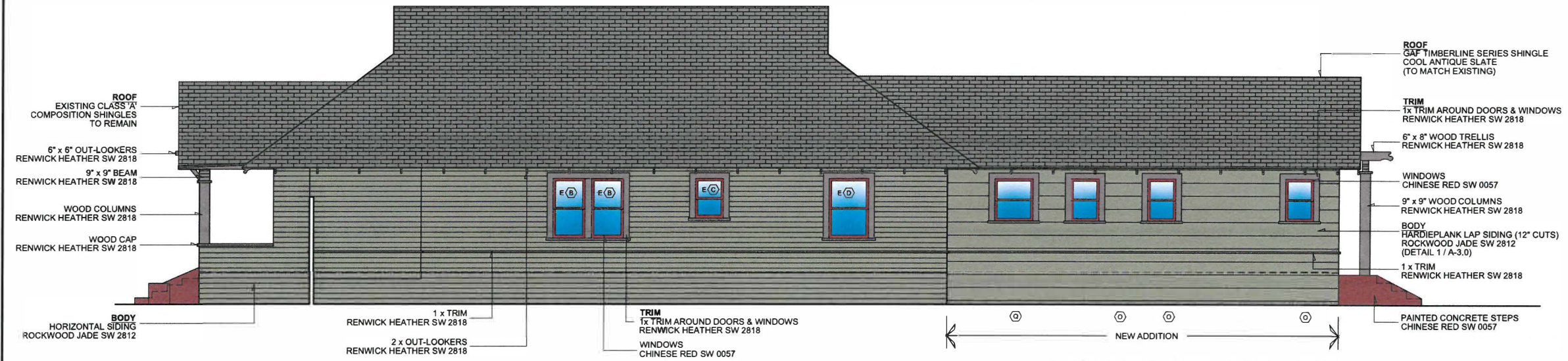
PROPOSED WEST ELEVATION Scale: 1/4"= 1'-0"
