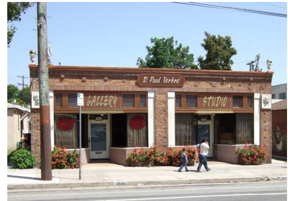
Large window openings bring activity and interest to the sidewalk and bulkheads at the ground plane communicate a sense of permanence for new structures.
