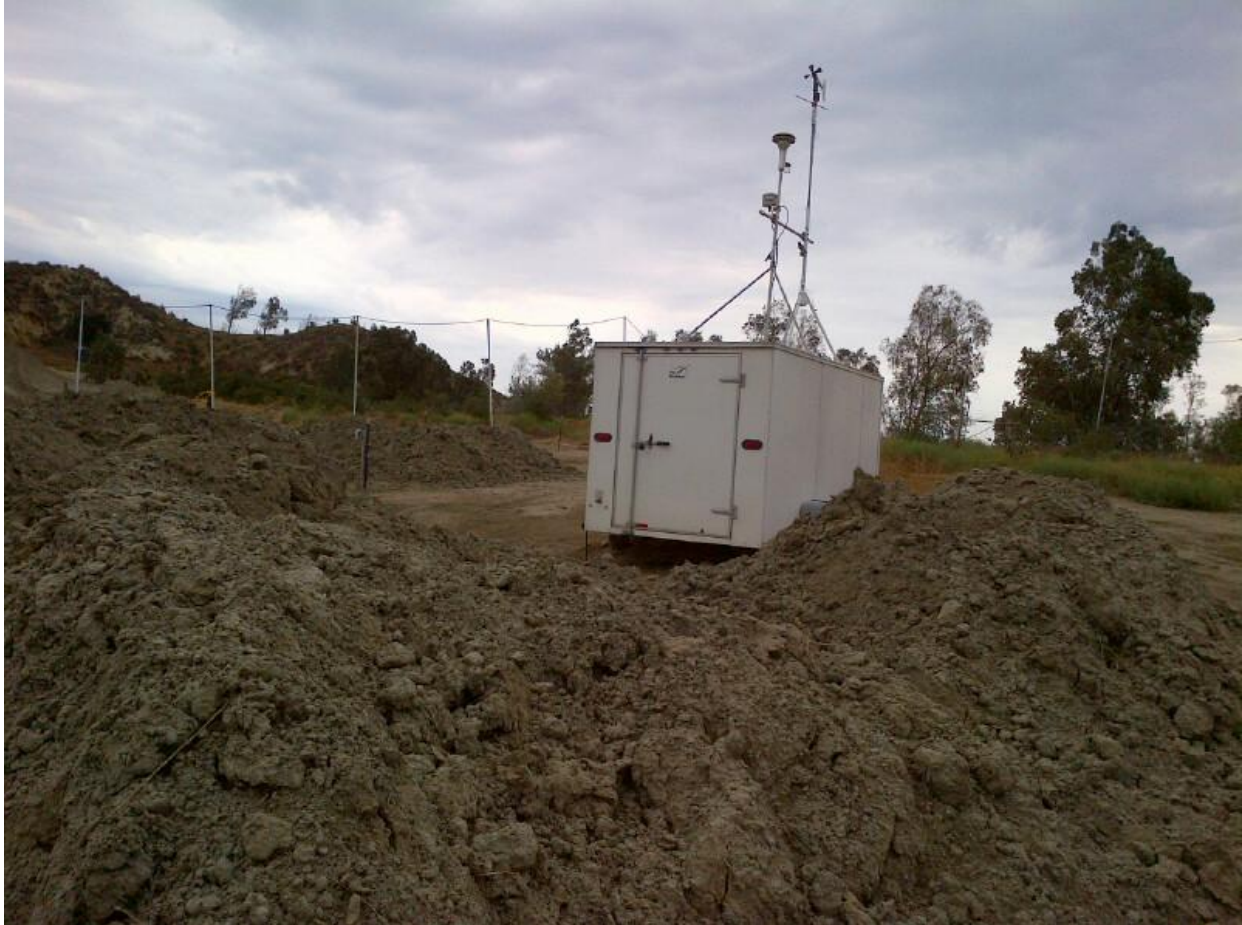
Figure 3-1. A re-vegetation project on the south berm of the Landfill has involved the movement and deposition of large quantities of soil, leading to short-term spikes in PM 10 concentrations recorded by the Landfill monitor.
