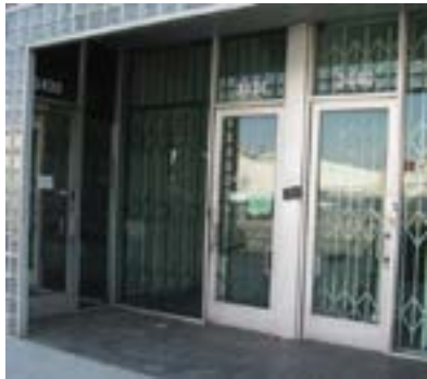
Interior security grilles are not visible during business hours and provide security, but do not create a blank wall, during non-business hours (4C.G4).
