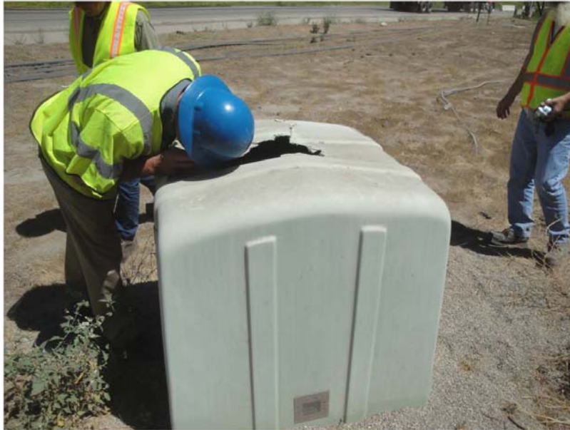
Photo 5: Damaged protective case for ground motion monitoring station
