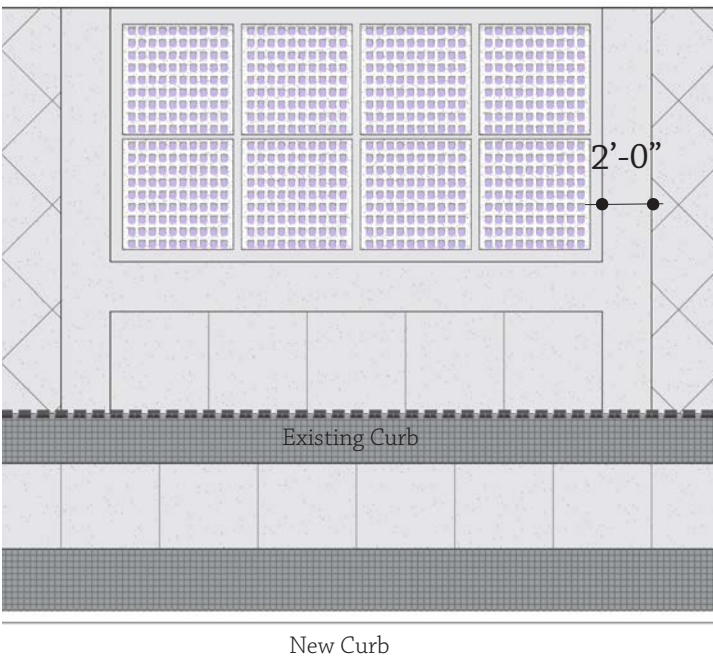
#4 West Side : Concrete Band at Existing Historic element when element runs only partway to back of curb
