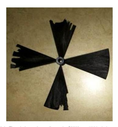
**Figure 2-1**. The wind speed propeller on the RM Young 5305 wind speed sensor at the Community site (Van Gogh School) suffered severe damage in January, causing significant loss of data.
