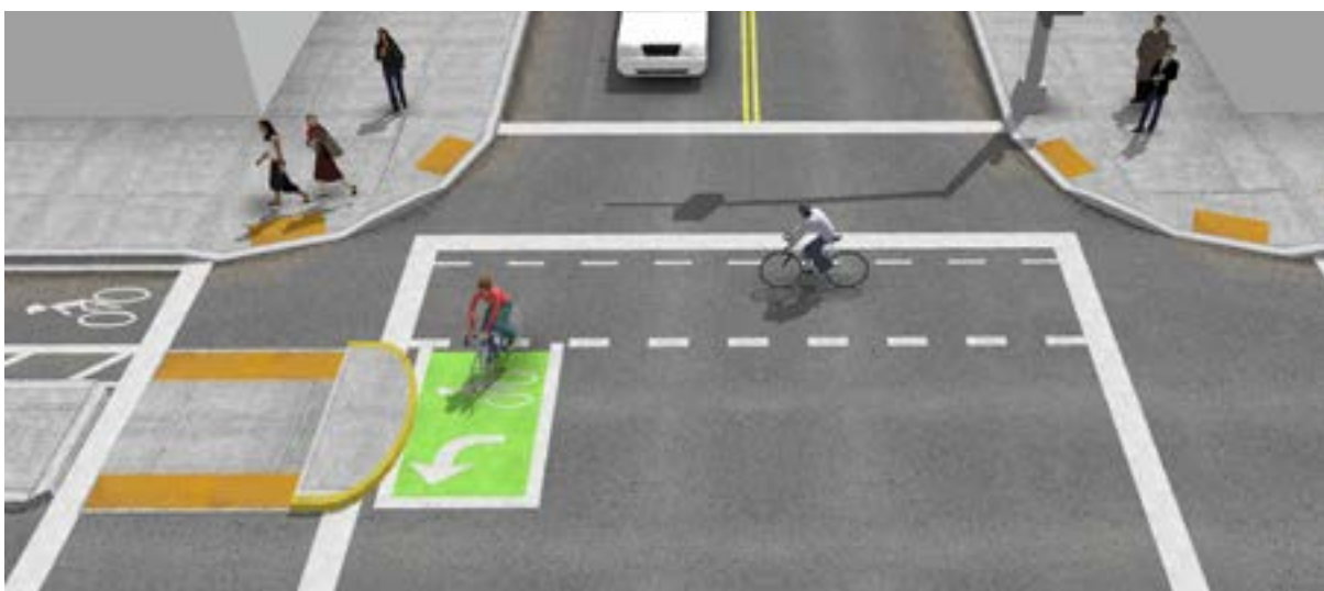
A Two-Stage Turn Queue Box separates turning bicyclists from through bicyclists.
