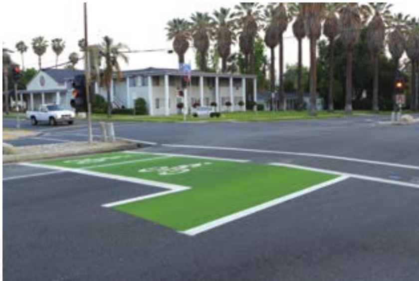
Coloring a Bicycle Box increases the box's visibility.
