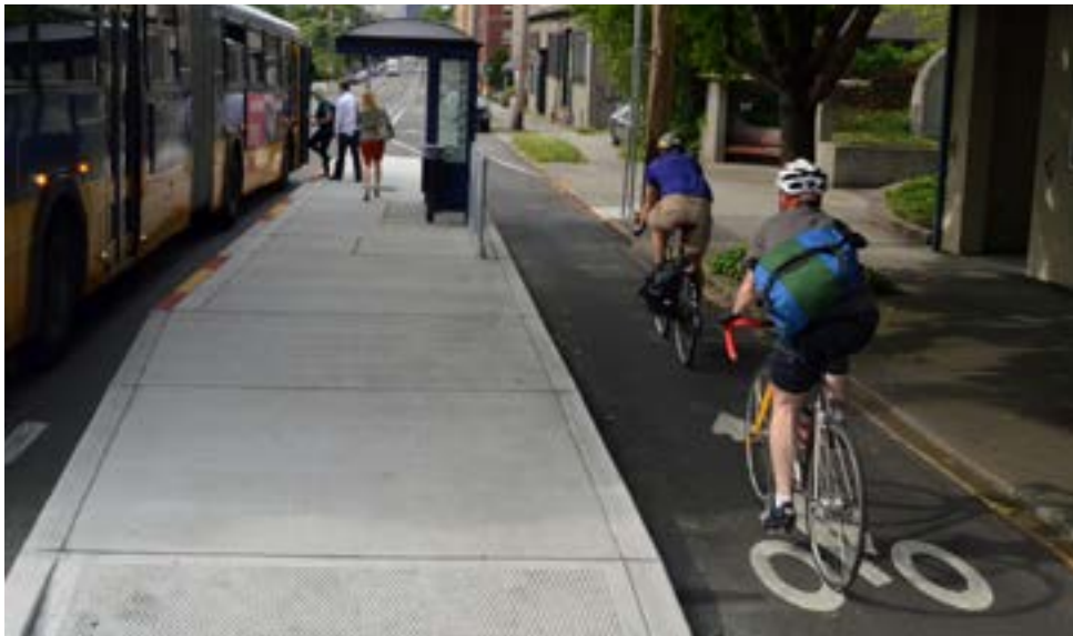
A median boarding island ensures access while allowing a protected cycle track to continue along an existing curbline. In this instance, the boarding island is accessed via a curb ramp (somewhat visible in the foreground) that adjoins the crosswalk.
