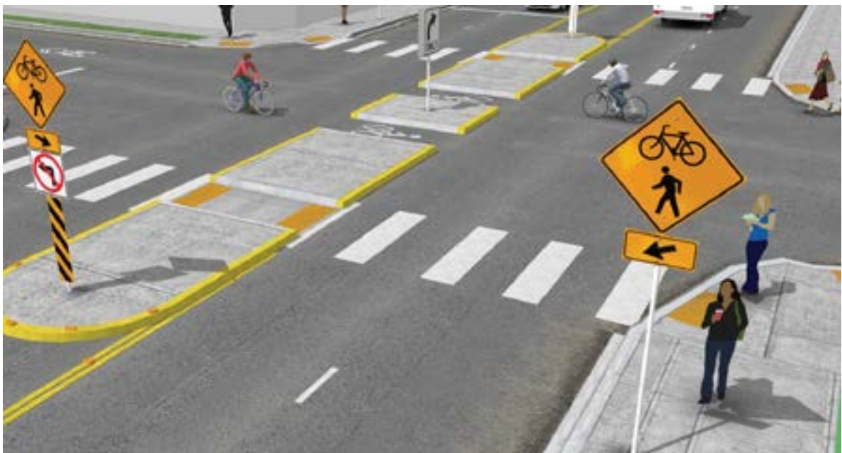
Crossing Refuge Islands should be marked by signs.
