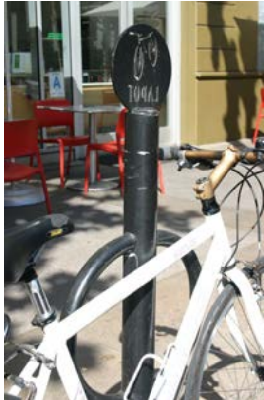
When an area with single-space parking meters is converted to multi-space pay stations, the decommissioned parking meter poles can be repurposed into bicycle racks.
