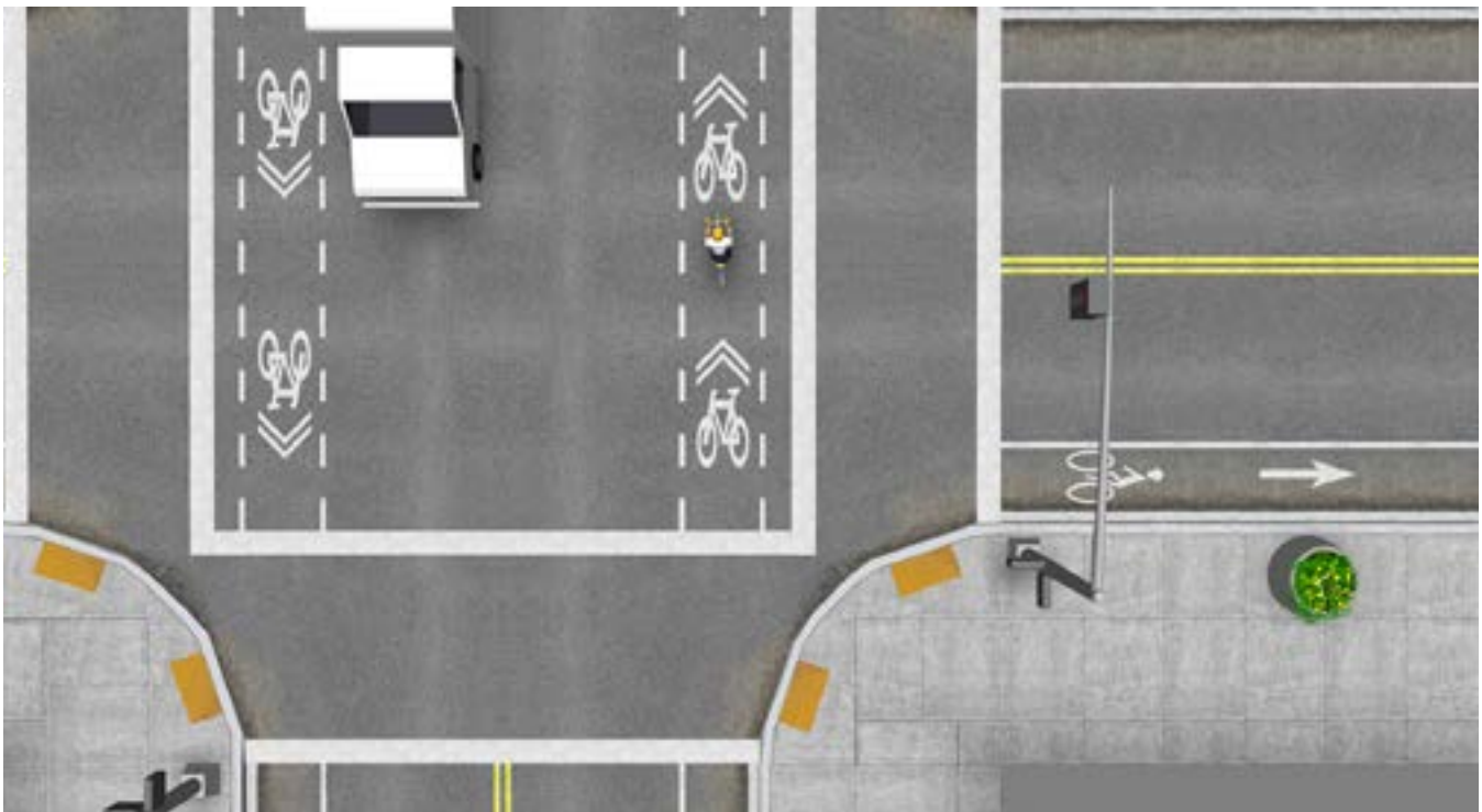
Bicycle Pavement Markings guide bicyclists through an intersection on a straight and direct path.
