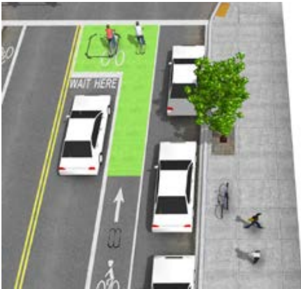
Bicycle Boxes enable bicyclists to position themselves to safely make left turns at an intersection.
