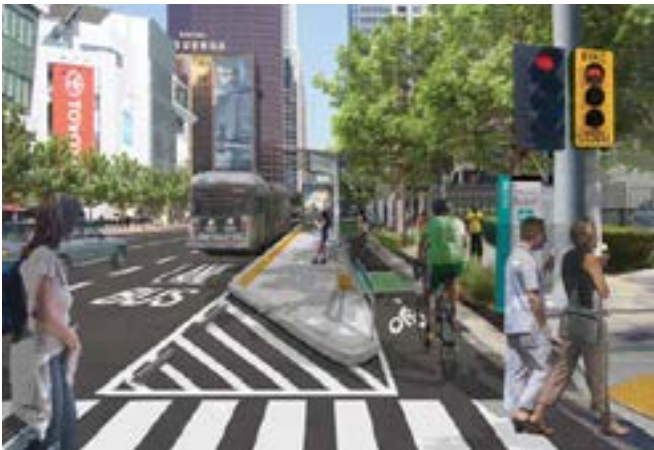
The Figueroa Street streetscape plan envisions protected bicycle lanes intermixing with bus boarding islands. (image courtesy of Melendrez)
