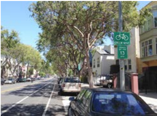
Bicycle Green Waves facilitate movement for bicycles while encouraging cars to travel at slower speeds..
