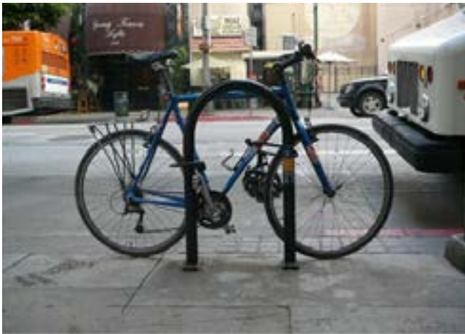
The “inverted-U” rack is the City’s accepted standard for on-street bicycle parking.
