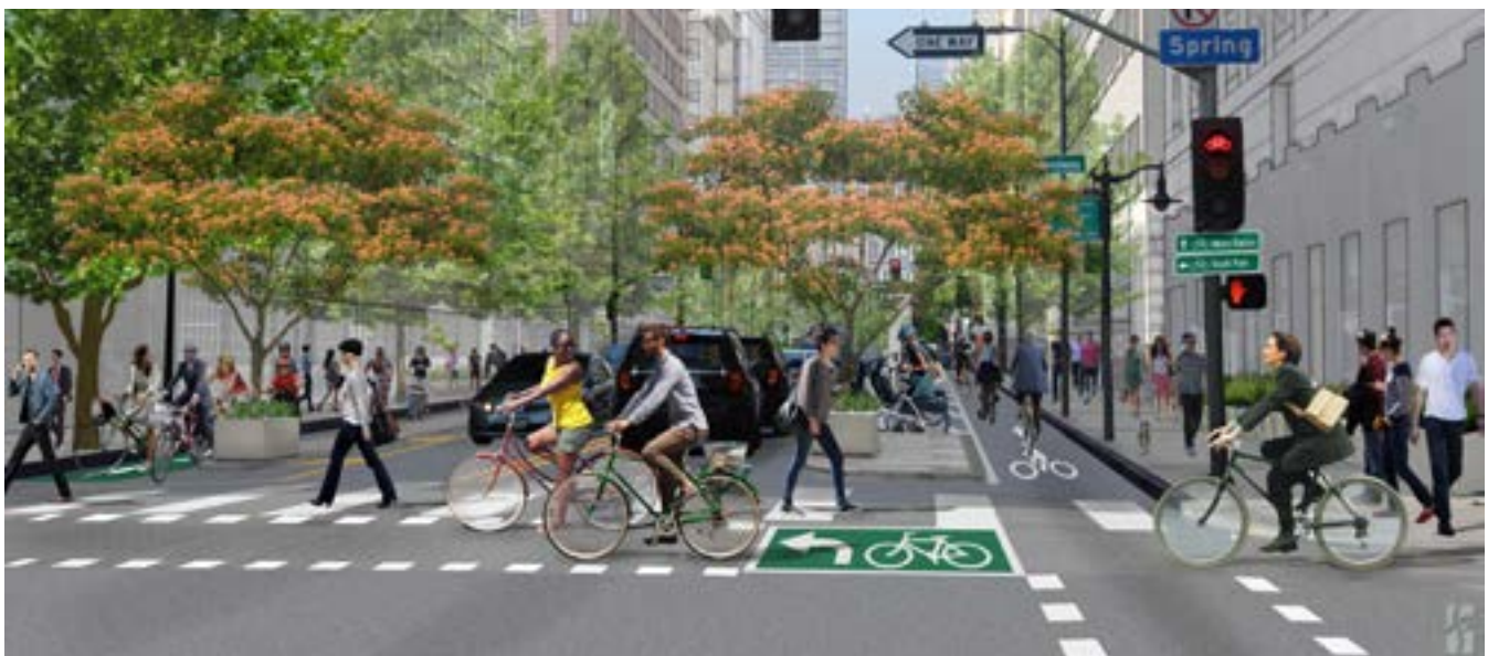
This conceptual rendering for 7th Street incorporates a wide buffered area that can accommodate non-car uses such as transit boarding islands, bikeshare stations, and bicycle parking corrals. (Image courtesy of Melendrez)
