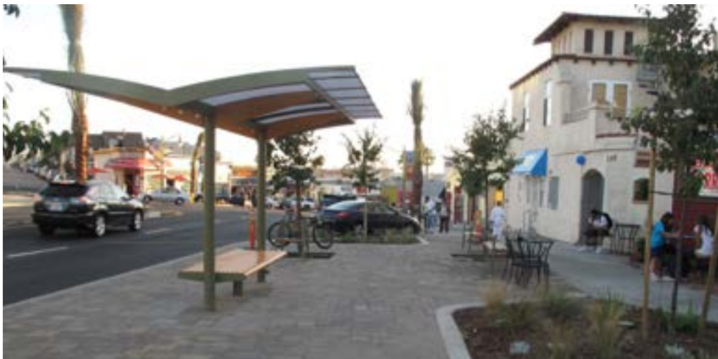
Locating Bus Stops midblock can allow riders to more easily access streetside shops and restaurants..
