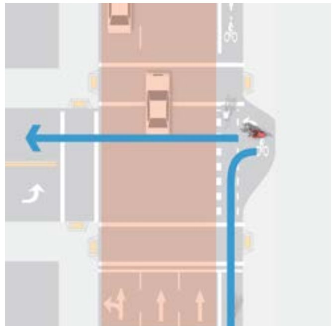
The pedestrian crosswalk can be realigned to create space for a Queue Box.
