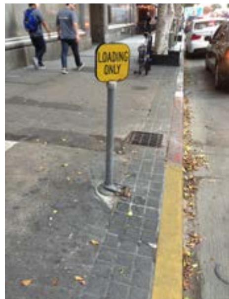
Loading and unloading zones should be designated by both signs and yellow-colored curbs..
