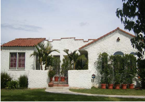
Historic stucco was generally smooth with subtle textures. Heavily textured stucco is inappropriate.
