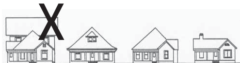
A complex roof form with many gables should not be simplified. Additions should never overpower the original structure, and should have the same roof form.
