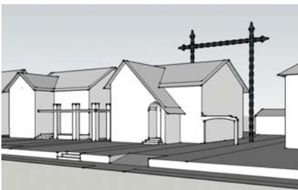
Additions should avoid breaking the side-plane and roof-plane of the existing house.
