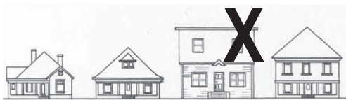
The home with the flat roof is inappropriate. The adjacent properties have pitched roofs -- any addition should take into consideration historic context. The bulk and massing of the second story, flat roof addition is out of scale with the other houses on the block.
