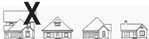
A complex roof form with many gables should not be simplified. Additions should never overpower the original structure, and should have the same roof form.
