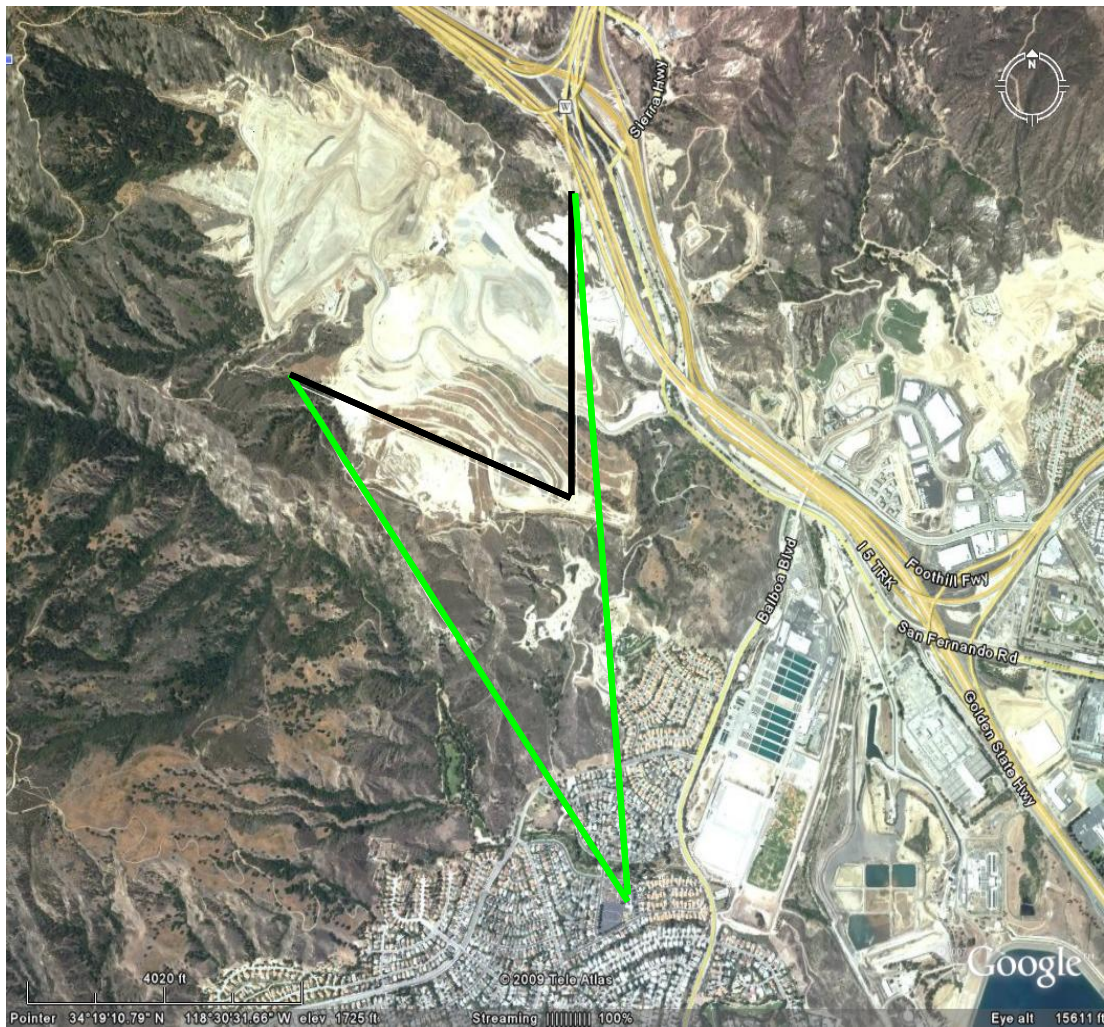
Figure 5-1. Aerial image of the Sunshine Canyon Landfill and the surrounding area, showing the wind direction sectors representing the landfill source used for selecting data for analysis from the Landfill monitor (in black) and the Community monitor (in green).
