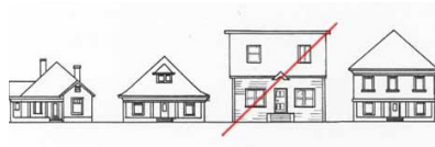
Standard 8e-8f example. 2nd floor addition is not to scale with the original structure and does not repeat original roofline.
