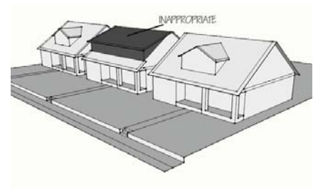
Altering the basic form of a visible roof is inappropriate.
