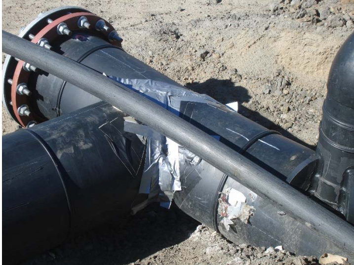
Photo 99: Broken Gas Collection Pipe at CC4 Slope: November 29, 2016
