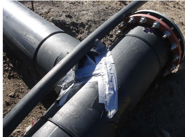
Photo 98: Broken Gas Collection Pipe at CC4 Slope: November 29, 2016
